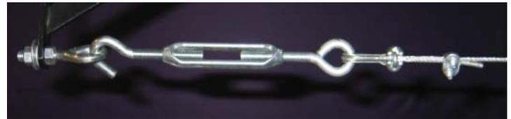
Cable is then fastened directly to the turnbuckle with a thimble and two cable clamps. Slack in the cable is taken up by the turnbuckle. If cable is still too loose after tightening the turnbuckle, loosen the cable, re-fasten cable to turnbuckle at a tighter position, and re-tighten the turnbuckle. Do not over-tighten the turnbuckle, we recommend no more than 100 lbs (445 Newtons) of tensile force.
