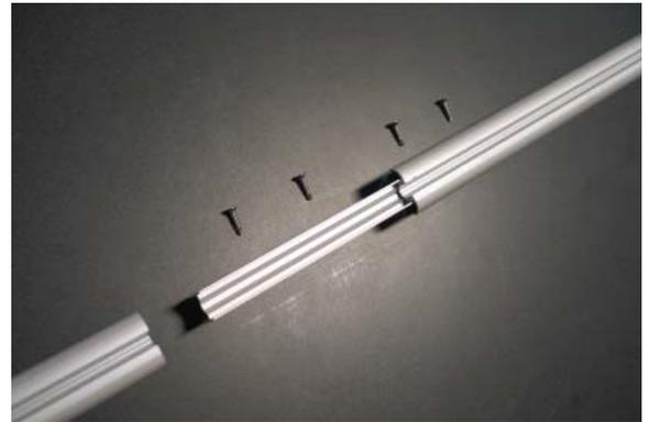
Insert the rest of the coupler into the other track. Be sure to get each section of track as close together as possible so that the coupler is not visible. Secure the coupler in the tracks with two screws for each track.
