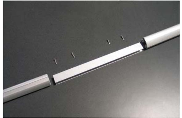
Coupler is inserted into one track about 6" (150mm) and secured with two screws. Screws are driven through the top of the track to secure coupler and track in place. Note: Use screws supplied.
