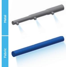
Traditional metal ductwork is heavy, rigid and can only disperse air through spaced out diffusers restricting airflow to localized areas.
