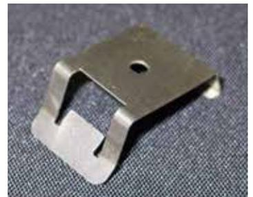
Optional T-Bar Clip: A T-Bar clip is riveted (by the installing contractor) to the Surface Mount clip. The U-Track is snapped to the Surface Mount clip and the bottom of the T-Bar ceiling support.
