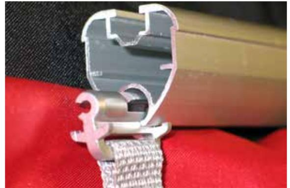
The Track Stop is used to keep shorter sections of DuctSox under slight tension. The screw is tightened into the bottom channel to lock the stop at locations where Gliders are to be locked in place.
