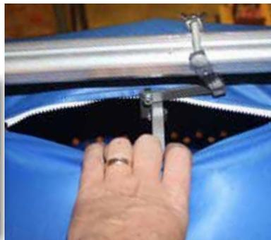
Top zipper, open (Note: In photo, tensioned section is on the right.)
