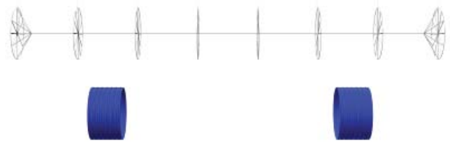
Fabric Located at Midpoint of Tensioned Sections
