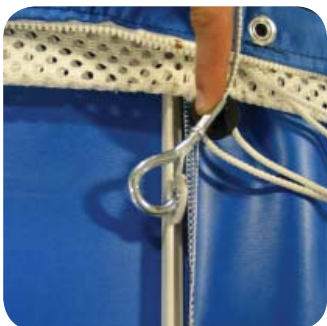
Lower Cable Connected to the ECR
