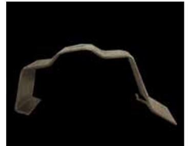
Optional T-Bar Clip: A T-Bar clip is riveted (by installing contractor) to the Surface Mount clip. The U-Track is snapped to the Surface Mount clip and the bottom of the T-Bar ceiling support.
