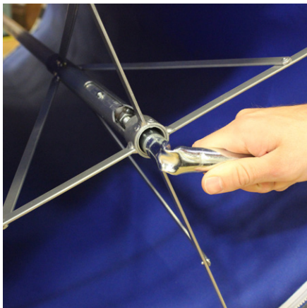
Interior Section CTR Tensioning
