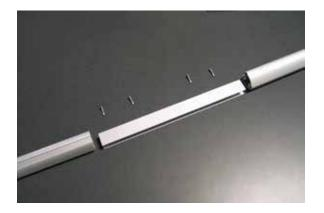
Coupler is inserted into one track about 6" (150mm) and secured with two screws. Screws are driven through the top of the track to secure coupler and track in place. Note: Use screws supplied.
