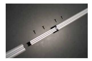
Insert the rest of the coupler into the other track. Be sure to get each section of track as close together as possible so that the coupler is not visible. Secure the coupler in the tracks with two screws for each track.
