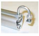
through an eyebolt attached to the ceiling. Be sure all of the threads of the square nuts are engaged to the U-bolt. The square nuts on the end of the U-bolt are slid into the top channel of the track. After U-bolt and cable are in their proper location the nuts (7/16"wrench) on the U-bolts must be tightened onto the track. A cable loop is created at the top of the track by the cable through the U-bolt clamp. After adjusting the track height trim excess cable as needed.
