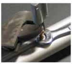
and cable are in their proper location the top nut (7/16"wrench) on the stud must be tightened onto the track while holding the stud with a pliers. After adjusting the track height trim excess cable as needed.
