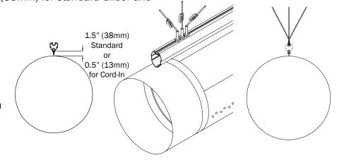
angles away from the sides of the track along with angled cables in-line with the track. See image above.
