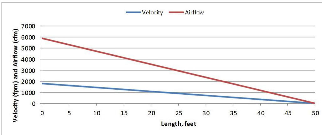
Figure 3. Velocity and airflow along duct length.
