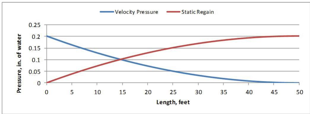
Figure 4. Velocity Pressure/Static Pressure Regain
