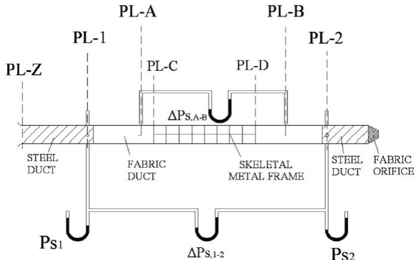
Figure 1. Schematic of testing setup with metal frame. Testing setup without metal frame would be depicted the same, but without “SKELETAL METAL FRAME”, PL-C AND PL-D.
