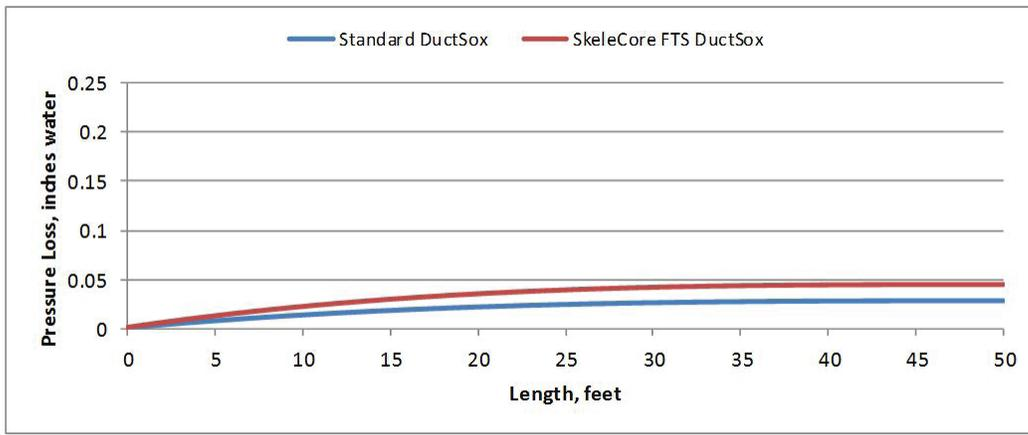
Figure 2. Pressure Loss for TAD systems with and without an internal metal frame.
