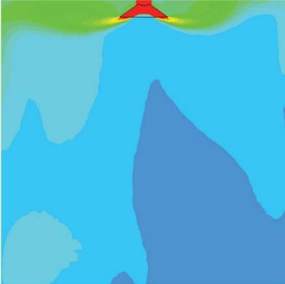
The uneven dispersion of a 4-way metal diffuser. Notice the inconsistencies in temperatures in the space.
