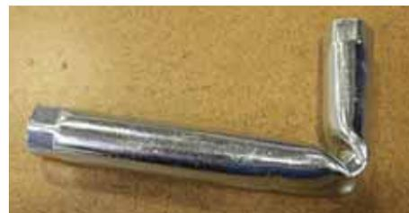
**CTR Wrench:** Used to adjust the CTR and apply tension to the fabric.
