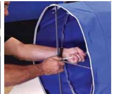
Bend Rod and secure in place
