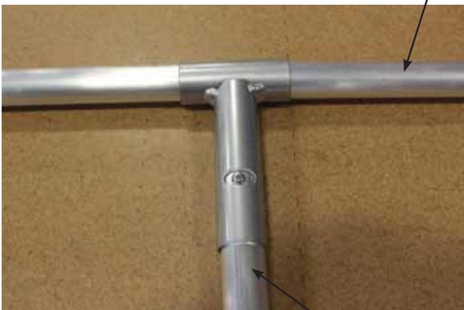
Tee Fitting Coupler Installed
