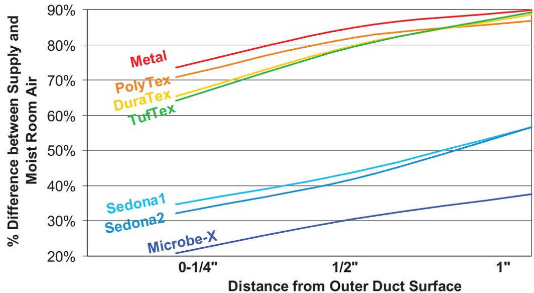
Figure 6: Temperature Difference (%) around Sample Surface
