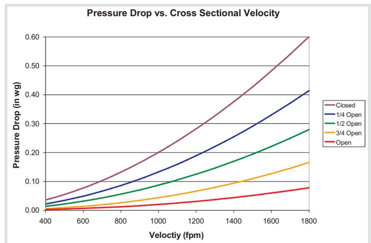
Fig. 4: Pressure drop vs. velocity
