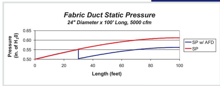
Figure 5: Static Pressure Regain
