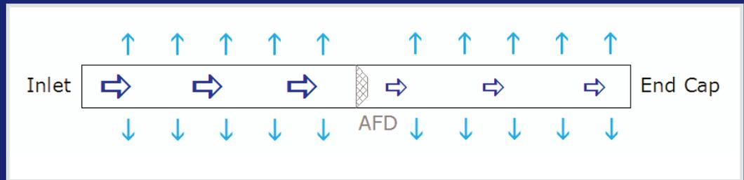
Fig. 9: AFD resists inflation velocity, resulting in smoother start-ups.
